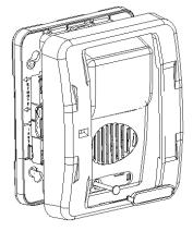
To remove bezel, grip both sides of bezel and pull in a download and outward motion.
