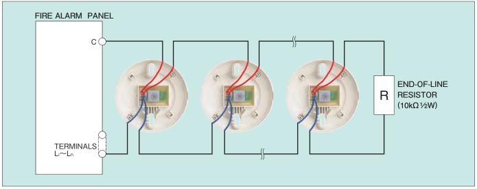
● Lead wire system ● Maximum number of detectors to be connected : No limit. ● External wire resistance : Less than 50 Ω / line
