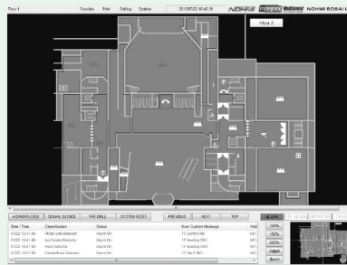
Floor plan under alarm condition
