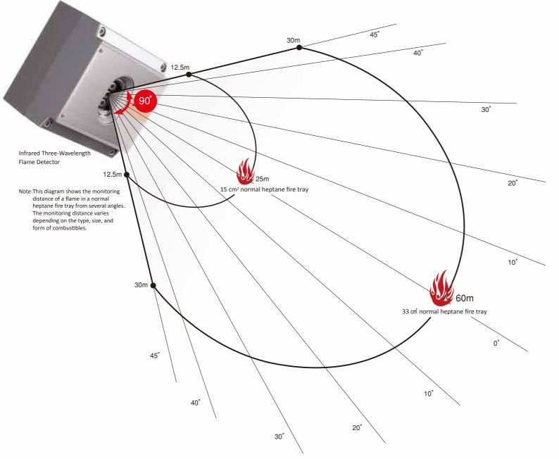
The PDCJ002-E detects the CO2 resonance radiation and flicker that are unique characteristics of flames. Despite its high sensitivity, the PDCJ002-E has fewer false alarm performance and can be installed under direct sunlight or artificial lighting such as sodium lamp, mercury lamp, fluorescent lamp, germicidal lamp, halogen lamp, etc.
