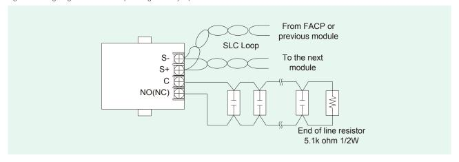
Figure 2: Wiring diagram in case of supervising Normally-Closed contact (Not recognized as NFPA Initiating Device Circuit)
